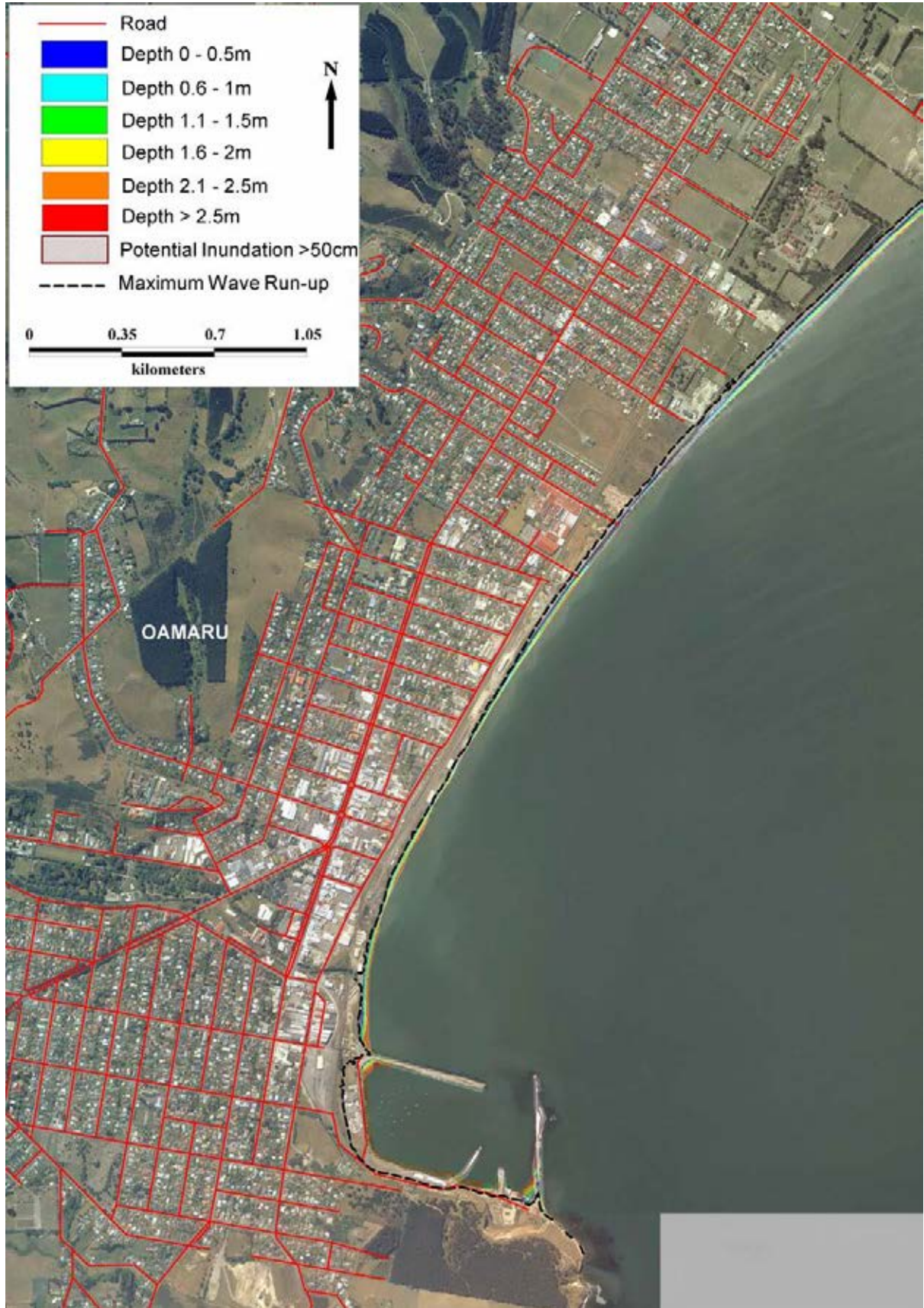
Figure A106. Maximum water depth for inundated land at Oamaru during a 1:500-year elevated sea level event at MHWS
