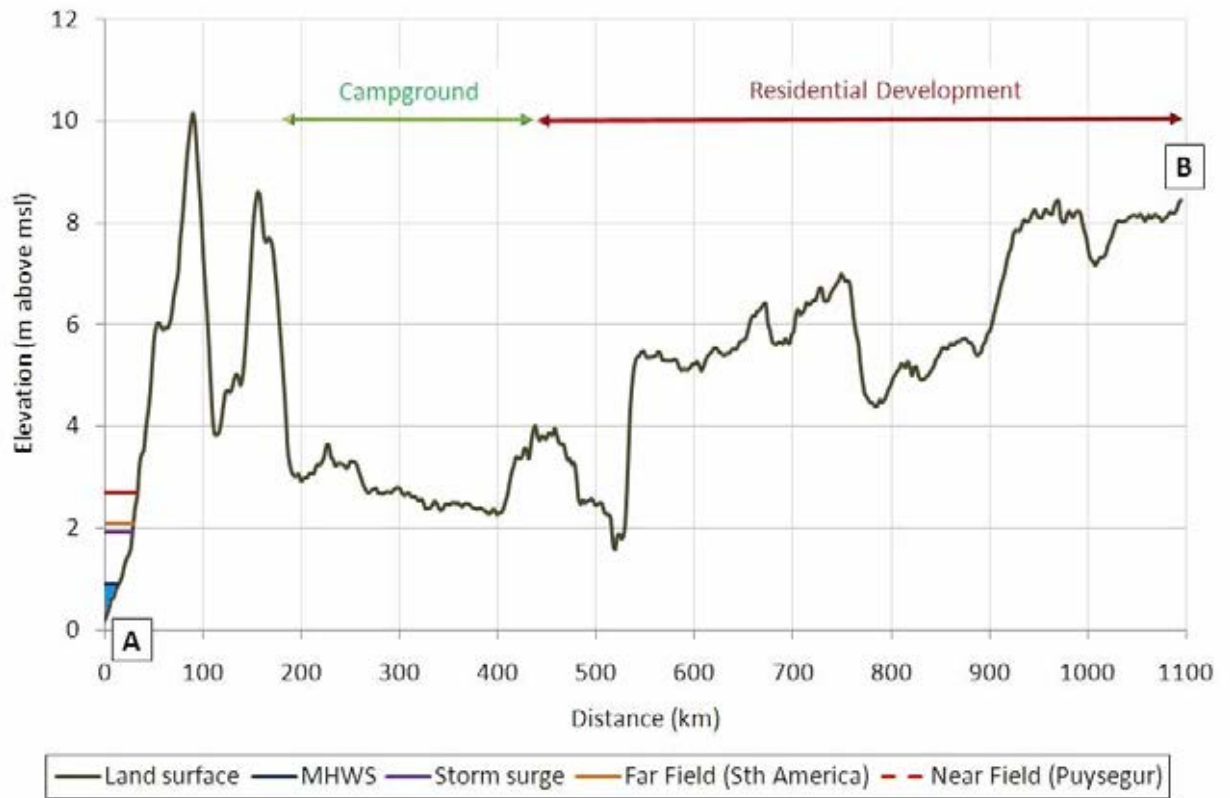
Figure A100. Cross section A-B through Waikouaiti, showing the greatest extent of run-up at the coast from 1:500-year South American and 1:600-year Puysegur tsunami, and a 1:500-year storm surge event
