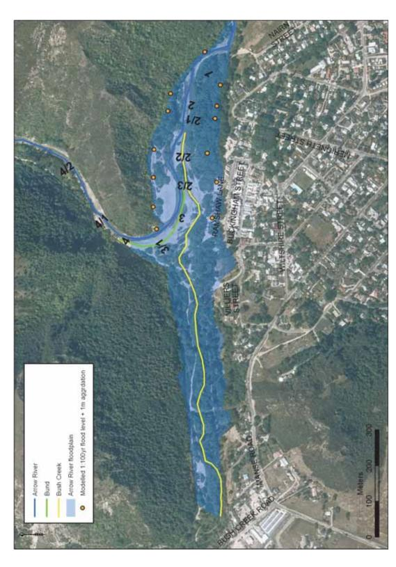
Arrow River/Bush Creek floodplain area, and the extent of the modelled 1:100-year flood level at each cross-section location Figure 12.
