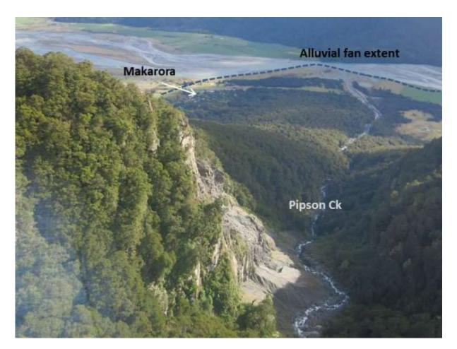
Figure 30. View down Pipson Creek, near Makarora (May 2015). The eroding cliffs in the foreground (and other cliffs upstream) contribute rock and sediment to the channel, which can mobilise into debris flows during high rainfall. Earthquake shaking is liable to cause extensive rockfall and landsliding into the creek.
