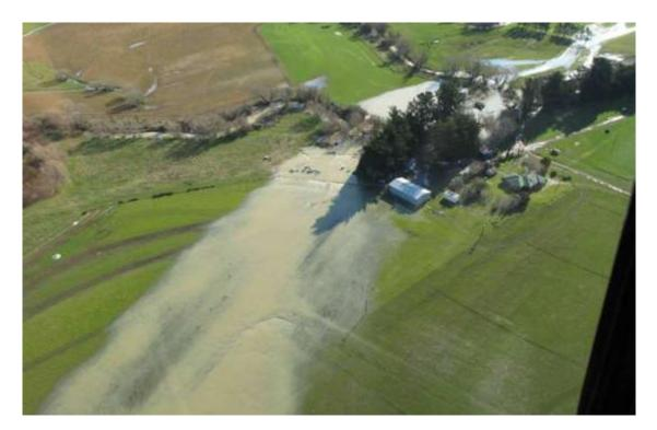
Figure 4. Avulsion of the Hororata River following fault movement during the September 2010 Darfield earthquake (photo courtesy D. Barrell, GNS Science)
