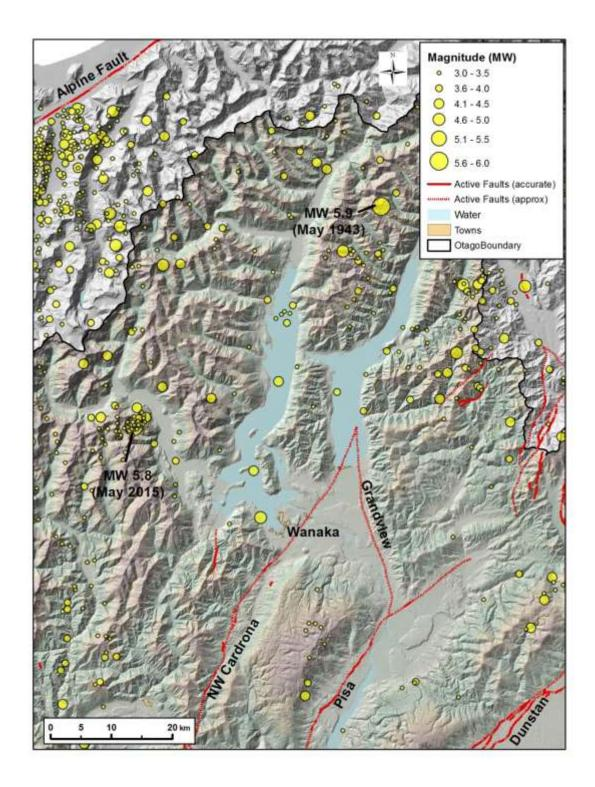
Figure 17. Historic seismicity in the West Otago area, with earthquakes larger than  $M_W$  3.0 from 1942 – July 2015. Two earthquakes larger than  $M_W$  5.5 have been recorded over that period. The highest concentration of earthquakes occurs towards the Alpine Fault in the northwest of the mapped area (data from GeoNet (accessed July 2015)).
