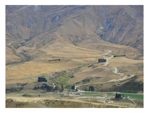
Figure 22. View towards the west across the Cardrona Valley. The Cardrona skifield access road runs lower right to upper left across the ridge. A visible, active trace of the NW Cardrona Fault is highlighted between the two arrows (photo April 2015).
