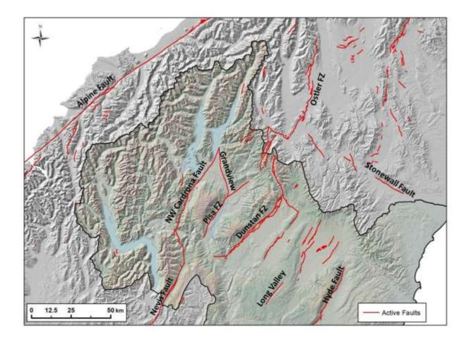
Figure 12. Active faults in West Otago and surrounding regions (from QMAP and GNS New Zealand Active Faults Database). Otago region is outlined.
