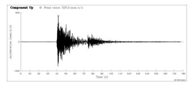
Figure 16. Seismograph record of vertical accelerations recorded at the Mt Aspiring National Park Visitor Centre during the May 4<sup>th</sup> 2015 earthquake (Figure 17). This event caused some stock to fall from shop shelves in Wanaka, with a peak acceleration of 0.054 g (image from GNS Science).
