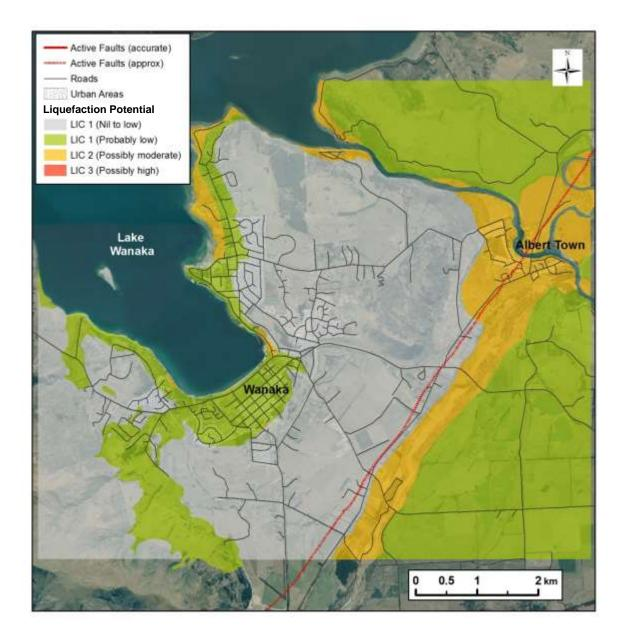
Figure 24. Map of liquefaction risk in the Wanaka area assessed by Tonkin & Taylor Ltd (2012) for the Queenstown Lakes District Council. The most susceptible layers are river courses and some lake-margin areas. The mapping is intended to guide the appropriate level of site investigation at the development stage, rather than assess the likelihood of liquefaction at a site.
