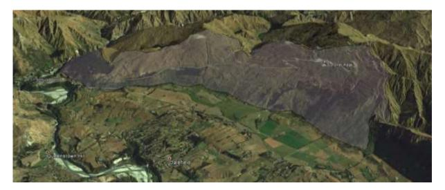
Figure 43. Oblique view showing outline of the Coronet Peak landslide, a large deep-seated schist landslide. The Shotover River runs along the left side of the image (Google Earth).
