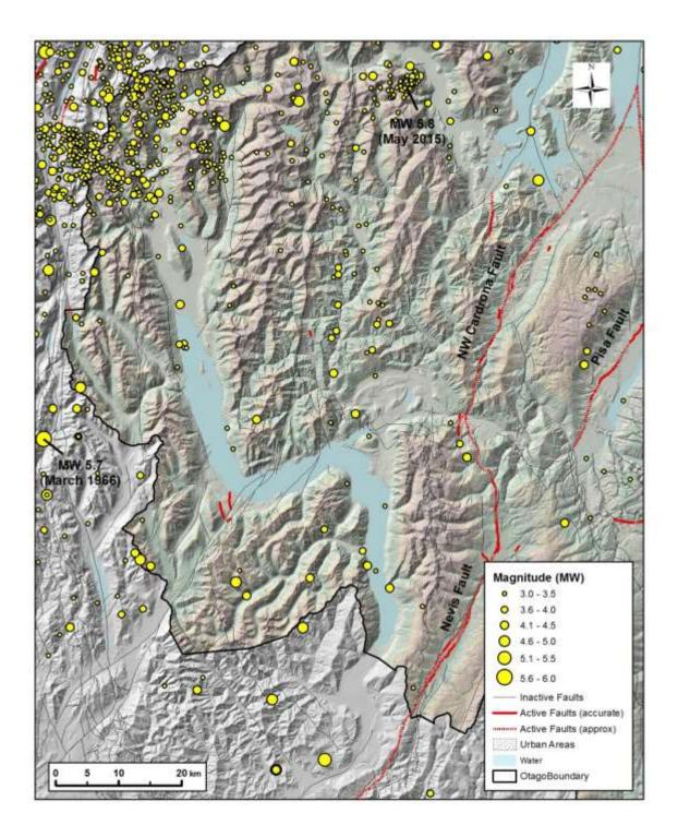
Figure 36. Historic seismicity in the Wakatipu area, with earthquakes larger than  $M_w$  3.0 from 1942 – July 2015. Two earthquakes larger than  $M_w$  5.5 have been recorded over that period (labelled). The highest concentration of earthquakes occurs towards the Alpine Fault in the northwest of the mapped area. The Alpine Fault is 80 km from downtown Queenstown (data from GeoNet (accessed July 2015)).
