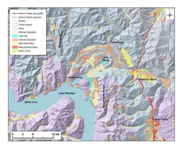
Figure 33. Geology of the Wakatipu area. The pale blues and purples are varying metamorphic grades of schist bedrock. Glacial (undifferentiated) and alluvial deposits occupy most of the valleys and lower hillslopes. Lake silts were deposited during a higher lake level. Isolated outcrops of the Tertiary Manuherikia sediments can be found east of the Nevis-Cardrona Fault Zone (modified from QMAP (Turnbull, 2000)).
