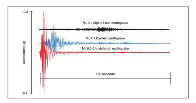
Figure 3. Seismographs from two Canterbury earthquakes as recorded in Christchurch in Sept. 2010 (blue line) and Feb. 2011 (red line). The black line is a synthetic seismograph predicting the level and duration of shaking recorded in Christchurch during a hypothetical Alpine Fault earthquake. The more distant but larger Alpine Fault event has less intense ground shaking, but continues for a much longer duration (Webb *et al.*, 2011).
