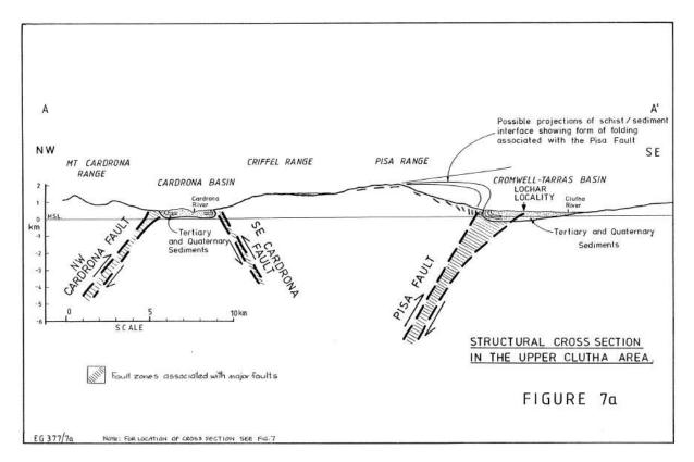
Figure 15. NW-SE oriented cross section through the Cardrona Valley and Cromwell Basin (marked on Figure 14) showing the orientation of major fault structures (Officers, 1984). Tertiary sediments remain preserved along the valley floors, but have been removed by erosion at higher elevations.
