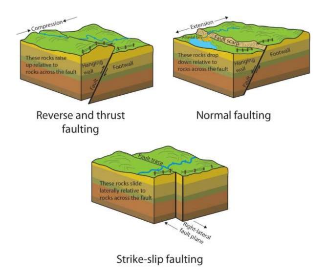
Figure 2. The main styles of faulting. Faults in western Otago are primarily reverse faults, reflecting the regional compression, whereas the Alpine Fault is a predominantly a strike-slip fault (from USDA National Park Service).
