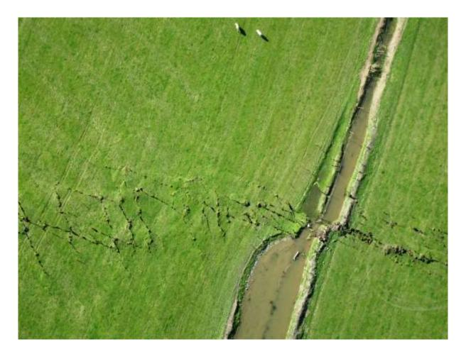
Figure 1. The surface trace of the Greendale Fault rupture cut across paddocks in the Canterbury Plains in September 2010 (photo courtesy M. Quigley). The ground moved up to 5.3 m laterally, but was expressed at the surface as a zone of distributed deformation up to 300 m wide, as seen in the network of shear structures (Quigley *et al.*, 2012).
