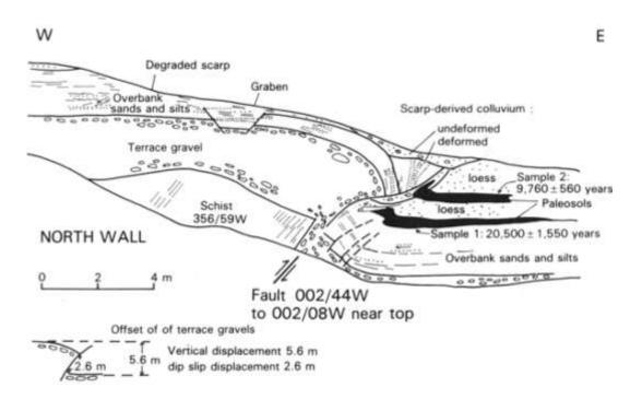
Figure 38. Cross section through the Kawarau trace of the Nevis Fault on the terrace above the Kawarau River. Evidence for three earthquakes can be seen in the deposits, which date to up to 23,000 years old (Beanland and Barrow-Hurlbert, 1998).
