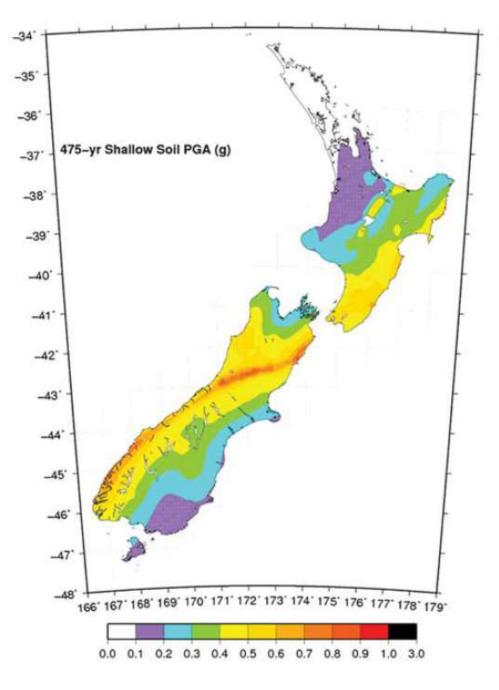
Figure 19. Probabilistic seismic hazard map for New Zealand (Stirling *et al.*, 2012). This map shows the maximum expected peak-ground acceleration (relative to gravity) expected over a 475-year period. The zone of red down the west of the South Island follows the Alpine Fault.
