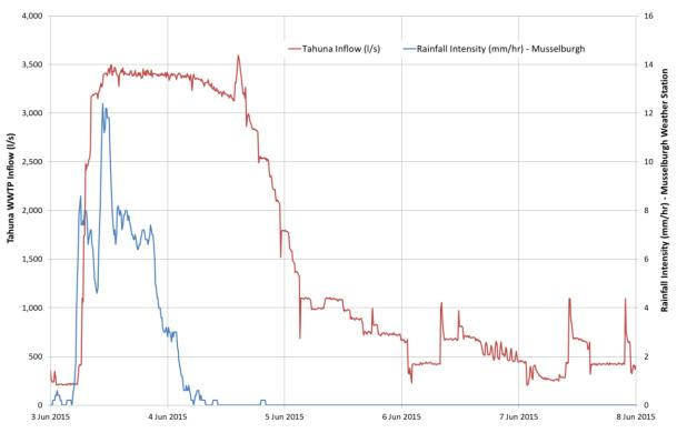
Figure 24. Inflow to the Tahuna wastewater treatment plant and rainfall intensity, 3/6/15 to 7/6/15.
