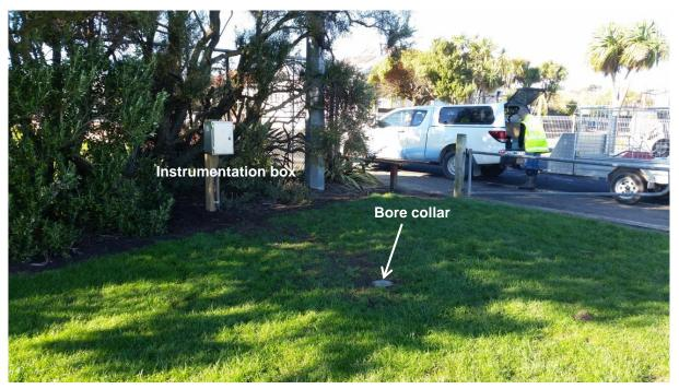
Figure 17. Typical example of an ORC bore installation, with bore collar and instrumentation box, at the Culling Park site.
