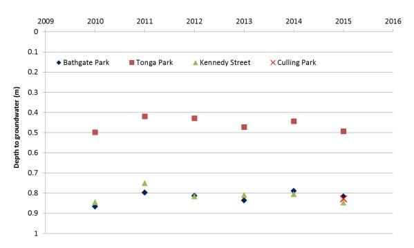
Figure 21. Median annual depth from the surveyed bore collar to groundwater level at ORC monitoring bores (complete years of record only). Note that the depth to groundwater at the Kennedy Street bore fluctuates by about 0.5 m as groundwater responds to the twice-daily ocean tidal cycles. It also rises and falls depending on the presence of low pressure storm systems and spring/neap tide monthly variations (see Figure 23).
