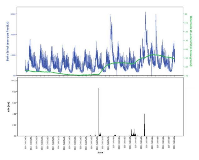
Figure 25. Graph of wastewater pipe flow at Botha Street (blue line), groundwater elevation at Lochend Street (green), and rainfall (black) between 24/12/12 and 6/1/13. Source: Fordyce (2013).
