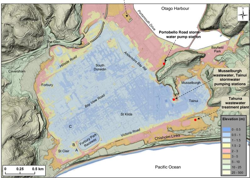
Figure 3. Topography and localities on the South Dunedin plain. Topographic features labelled A-C are shown in Figure 20. Background image is Dunedin City LiDAR, flown 2009, and coloured according to elevation. Elevation is in metres above MSL (mean sea level).
