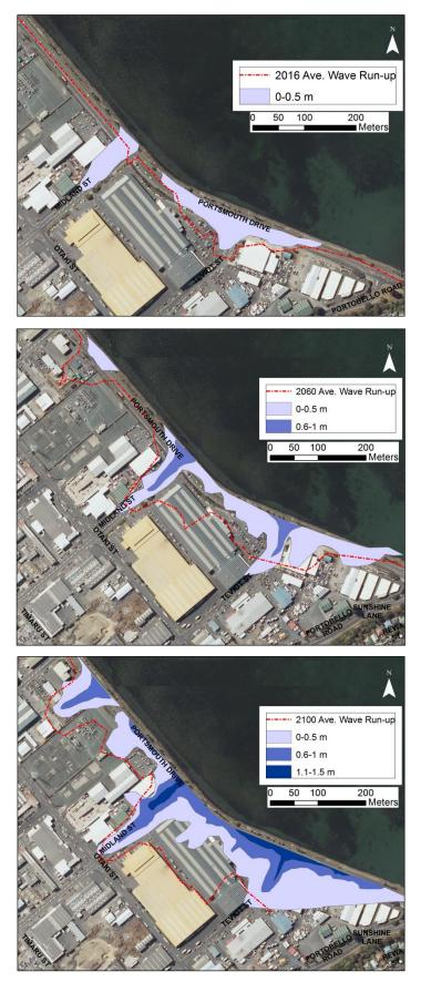
Figure 44. Likely extent and depth of inundation (shaded areas) and maximum extent of wave run-up (red-line) from Otago Harbour during a 1:20-year storm surge event at MHWS. Current sea level (top), 0.3 m mean sea level rise (middle), and 0.5 m rise (lower). Ave = average.
