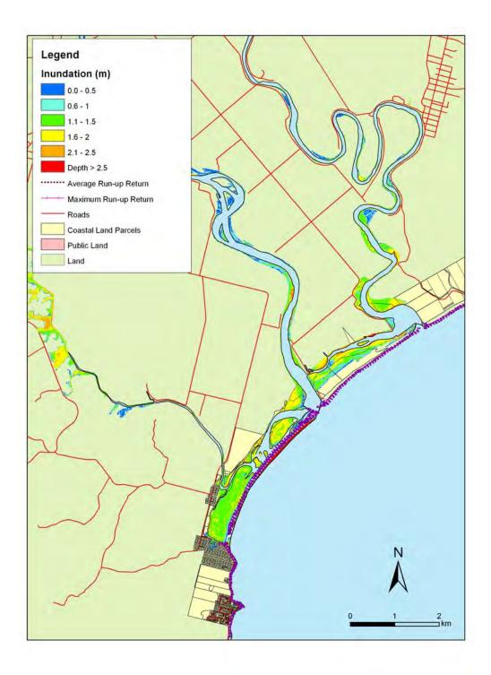
**Figure 5.45:** Kaka Point and Clutha - 1:20 year sea level event at MLOS + 0.5m: Maximum water depth for inundated land and the mean and maximum wave run-up.
