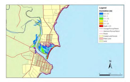
**Figure 5.188:** Taranui and Kakanui - 1:500 year sea level event at MLOS + 0.3m: Maximum water depth for inundated land and the mean and maximum wave run-up.
