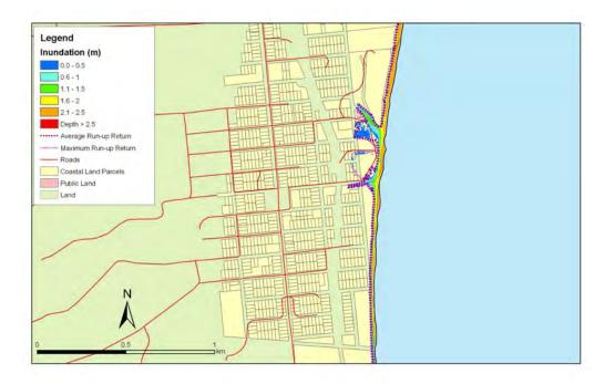
**Figure 5.176:** Hampden - 1:500 year sea level event at MLOS + 0.3m: Maximum water depth for inundated land and the mean and maximum wave run-up.
