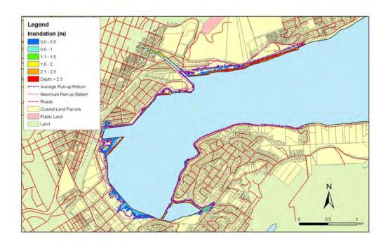
**Figure 5.116.** Dunedin Harbour - 1:500 year sea level event at MLOS + 0.3m: Maximum water depth for inundated land and the mean and maximum wave run-up.
