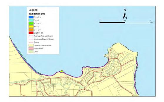
Figure 5.160: Moeraki - 1:500 year sea level event at present MLOS: Maximum water depth for inundated land and the mean and maximum wave run-up.
