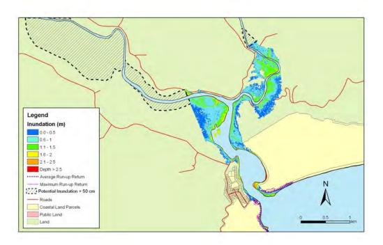
**Figure 5.23:** Papatowai - 1:100 year sea level event at MLOS + 0.5m: Maximum water depth for inundated land and the mean and maximum wave run-up.
