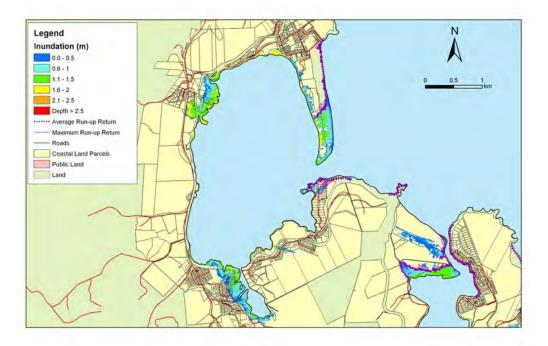
**Figure 5.143:** Warrington and Blueskin Bay - 1:100 year sea level event at MLOS + 0.5m: Maximum water depth for inundated land and the mean and maximum wave run-up.
