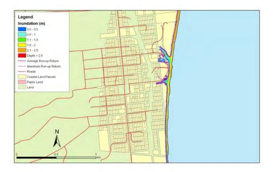
**Figure 5.174:** Hampden - 1:50 year sea level event at MLOS + 0.3m: Maximum water depth for inundated land and the mean and maximum wave run-up.
