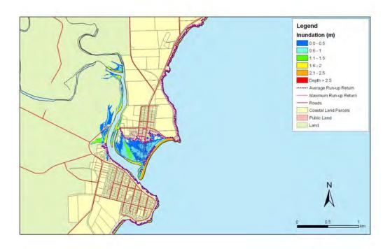
**Figure 5.187:** Taranui and Kakanui - 1:100 year sea level event at MLOS + 0.3m: Maximum water depth for inundated land and the mean and maximum wave run-up.
