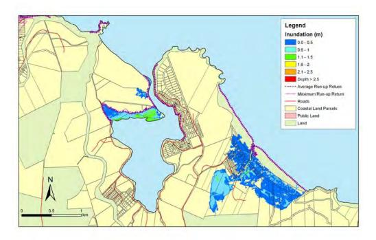
**Figure 5.126:** Long Beach and Purakanui - 1:50 year sea level event at MLOS + 0.3m: Maximum water depth for inundated land and the mean and maximum wave run-up.
