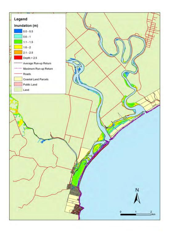
**Figure 5.43:** Kaka Point and Clutha - 1:100 year sea level event at MLOS + 0.3m: Maximum water depth for inundated land and the mean and maximum wave run-up.
