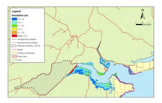
**Figure 5.29:** Catlins - 1:20 year sea level event at MLOS + 0.3m: Maximum water depth for inundated land and the mean and maximum wave run-up.
