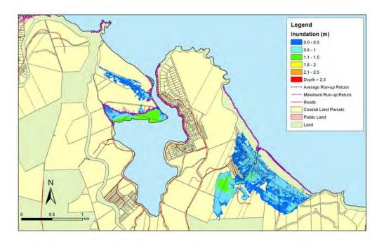
**Figure 5.131:** Long Beach and Purakanui - 1:100 year sea level event at MLOS + 0.5m: Maximum water depth for inundated land and the mean and maximum wave run-up.
