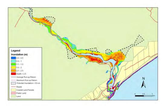
**Figure 5.58:** Toko Mouth - 1:50 year sea level event at MLOS + 0.5m: Maximum water depth for inundated land and the mean and maximum wave run-up.
