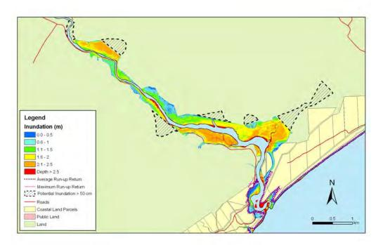
**Figure 5.53:** Toko Mouth - 1:20 year sea level event at MLOS + 0.3m: Maximum water depth for inundated land and the mean and maximum wave run-up.
