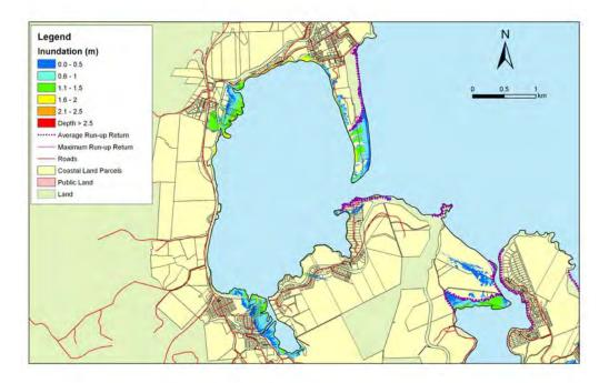
**Figure 5.141:** Warrington and Blueskin Bay - 1:20 year sea level event at MLOS + 0.5m: Maximum water depth for inundated land and the mean and maximum wave run-up.
