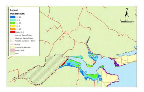
Figure 5.33: Catlins - 1:20 year sea level event at MLOS + 0.5m: Maximum water depth for inundated land and the mean and maximum wave run-up.
