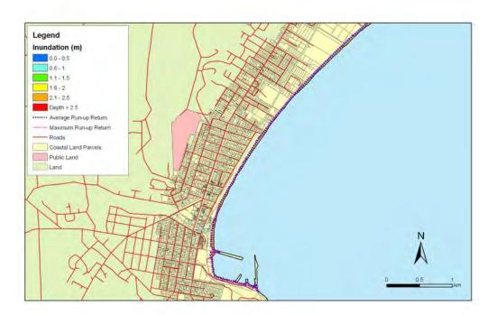
**Figure 5.198:** Oamaru - 1:50 year sea level event at MLOS + 0.3m: Maximum water depth for inundated land and the mean and maximum wave run-up.
