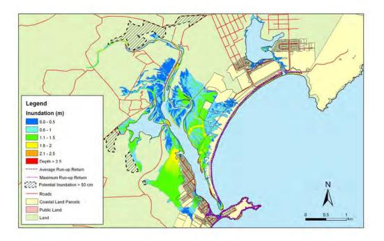
Figure 5.148: Karitane - 1:500 year sea level event at present MLOS: Maximum water depth for inundated land and the mean and maximum wave run-up.
