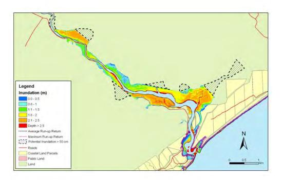
**Figure 5.54:** Toko Mouth - 1:50 year sea level event at MLOS + 0.3m: Maximum water depth for inundated land and the mean and maximum wave run-up.
