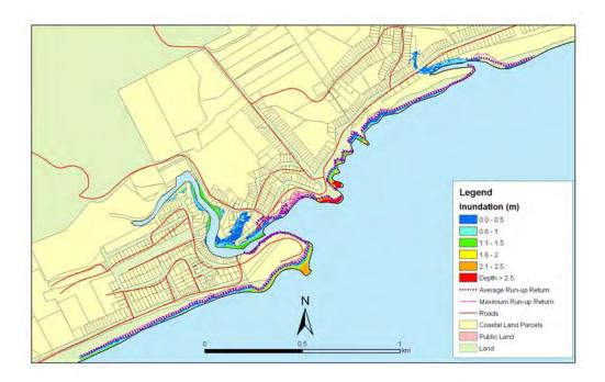
**Figure 5.82:** Brighton - 1:50 year sea level event at MLOS + 0.5m: Maximum water depth for inundated land and the mean and maximum wave run-up.
