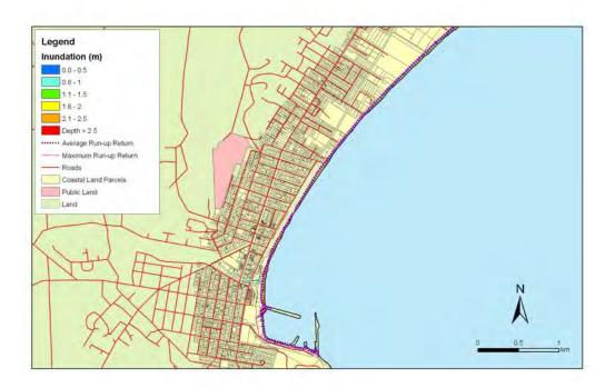
**Figure 5.199:** Oamaru - 1:100 year sea level event at MLOS + 0.3m: Maximum water depth for inundated land and the mean and maximum wave run-up.
