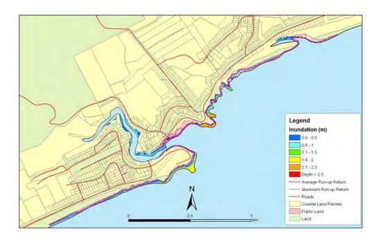
**Figure 5.74:** Brighton - 1:50 year sea level event at present MLOS: Maximum water depth for inundated land and the mean and maximum wave run-up.
