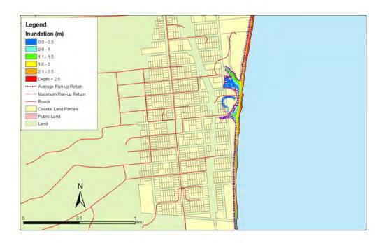
**Figure 5.180:** Hampden - 1:500 year sea level event at MLOS + 0.5m: Maximum water depth for inundated land and the mean and maximum wave run-up
