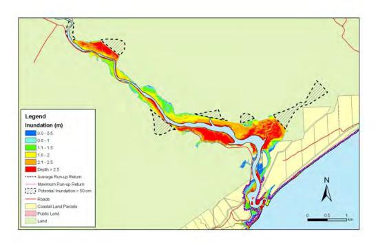
**Figure 5.60:** Toko Mouth - 1:500 year sea level event at MLOS + 0.5m: Maximum water depth for inundated land and the mean and maximum wave run-up.
