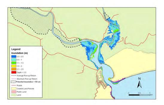
**Figure 5.18:** Papatowai - 1:50 year sea level event at MLOS + 0.3m: Maximum water depth for inundated land and the mean and maximum wave run-up.
