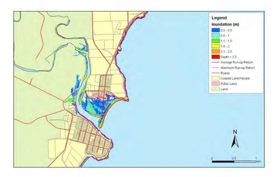
**Figure 5.186:** Taranui and Kakanui - 1:50 year sea level event at MLOS + 0.3m: Maximum water depth for inundated land and the mean and maximum wave run-up.
