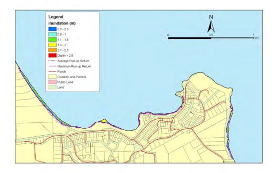
**Figure 5.164:** Moeraki - 1:500 year sea level event at MLOS + 0.3m: Maximum water depth for inundated land and the mean and maximum wave run-up.
