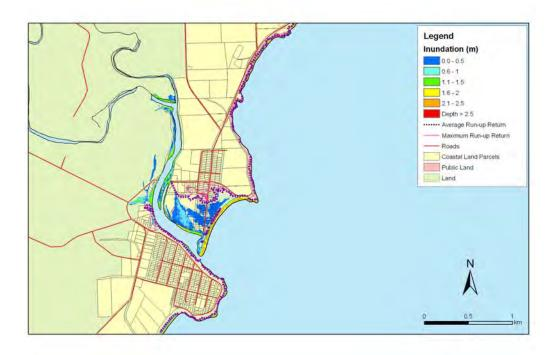
**Figure 5.189:** Taranui and Kakanui - 1:20 year sea level event at MLOS + 0.5m: Maximum water depth for inundated land and the mean and maximum wave run-up.
