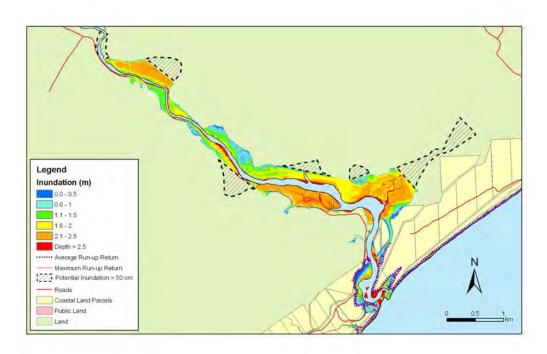
**Figure 5.55:** Toko Mouth - 1:100 year sea level event at MLOS + 0.3m: Maximum water depth for inundated land and the mean and maximum wave run-up.
