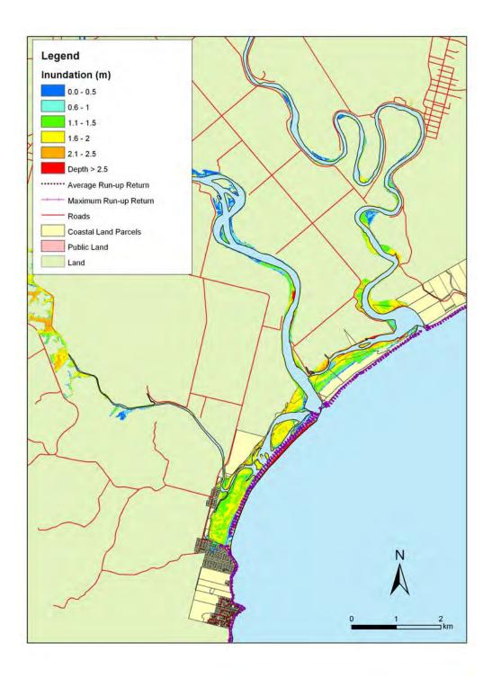
**Figure 5.47:** Kaka Point and Clutha - 1:100 year sea level event at MLOS + 0.5m: Maximum water depth for inundated land and the mean and maximum wave run-up.
