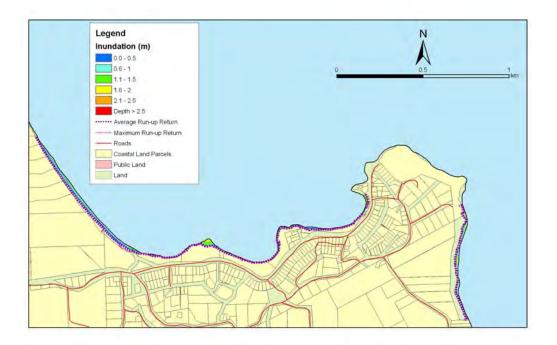
Figure 5.159: Moeraki - 1:100 year sea level event at present MLOS: Maximum water depth for inundated land and the mean and maximum wave run-up.
