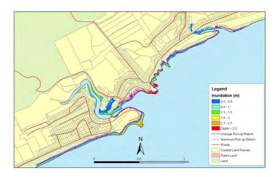
**Figure 5.80:** Brighton - 1:500 year sea level event at MLOS + 0.3m: Maximum water depth for inundated land and the mean and maximum wave run-up.
