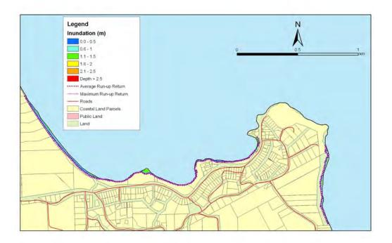
Figure 5.157: Moeraki - 1:20 year sea level event at present MLOS: Maximum water depth for inundated land and the mean and maximum wave run-up.
