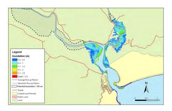
**Figure 5.19:** Papatowai - 1:100 year sea level event at MLOS + 0.3m: Maximum water depth for inundated land and the mean and maximum wave run-up.
