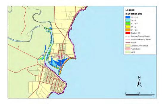
**Figure 5.182:** Taranui and Kakanui - 1:50 year sea level event at present MLOS: Maximum water depth for inundated land and the mean and maximum wave run-up.
