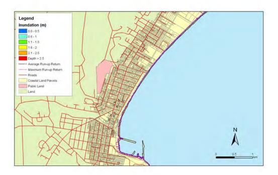
Figure 5.193: Oamaru - 1:20 year sea level event at present MLOS: Maximum water depth for inundated land and the mean and maximum wave run-up.
