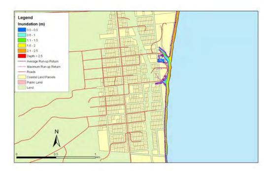
**Figure 5.175:** Hampden - 1:100 year sea level event at MLOS + 0.3m: Maximum water depth for inundated land and the mean and maximum wave run-up.
