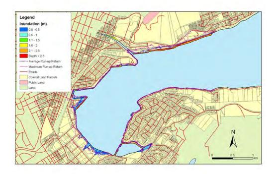
**Figure 5.114:** Dunedin Harbour - 1:50 year sea level event at MLOS + 0.3m: Maximum water depth for inundated land and the mean and maximum wave run-up.
