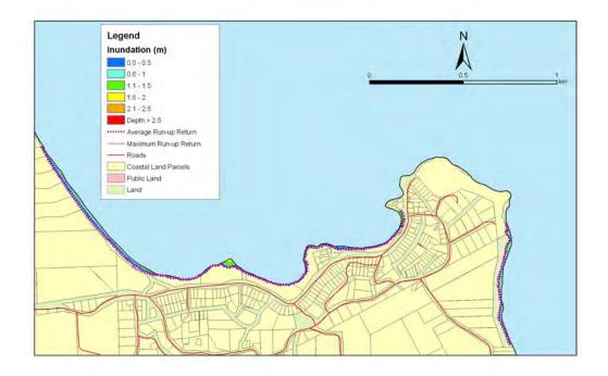
Figure 5.158: Moeraki - 1:50 year sea level event at present MLOS: Maximum water depth for inundated land and the mean and maximum wave run-up.
