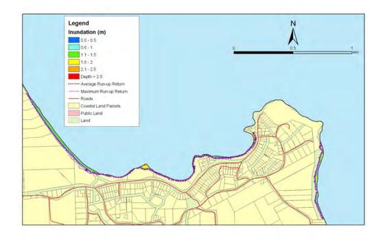
**Figure 5.166:** Moeraki - 1:50 year sea level event at MLOS + 0.5m: Maximum water depth for inundated land and the mean and maximum wave run-up.
