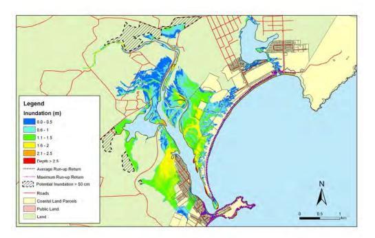
**Figure 5.151:** Karitane - 1:100 year sea level event at MLOS + 0.3m: Maximum water depth for inundated land and the mean and maximum wave run-up.
