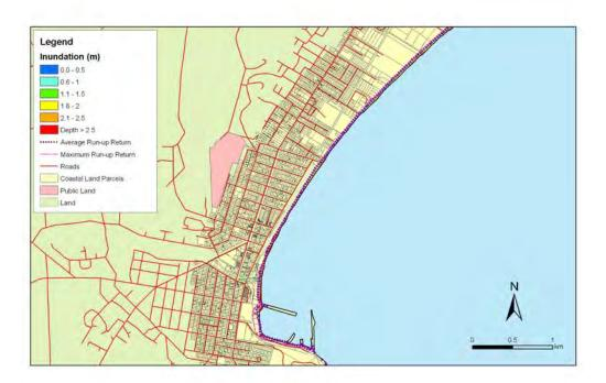
**Figure 5.202:** Oamaru - 1:50 year sea level event at MLOS + 0.5m: Maximum water depth for inundated land and the mean and maximum wave run-up.
