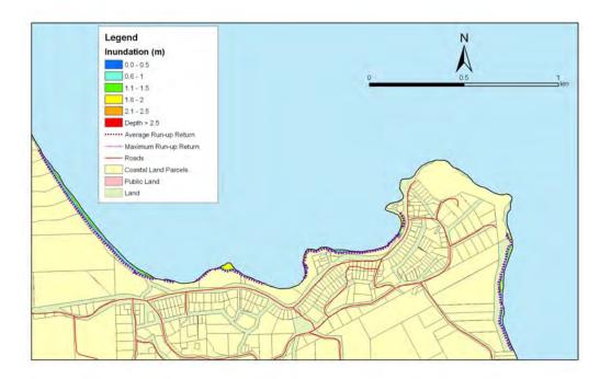
**Figure 5.163:** Moeraki - 1:100 year sea level event at MLOS + 0.3m: Maximum water depth for inundated land and the mean and maximum wave run-up.
