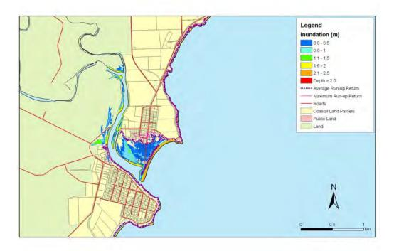
**Figure 5.184:** Taranui and Kakanui - 1:500 year sea level event at present MLOS: Maximum water depth for inundated land and the mean and maximum wave run-up.
