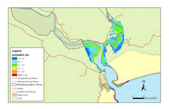
**Figure 5.24:** Papatowai - 1:500 year sea level event at MLOS + 0.5m: Maximum water depth for inundated land and the mean and maximum wave run-up.
