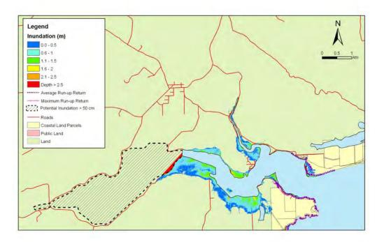
**Figure 5.30:** Catlins - 1:50 year sea level event at MLOS + 0.3m: Maximum water depth for inundated land and the mean and maximum wave run-up.
