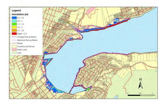
**Figure 5.120:** Dunedin Harbour - 1:500 year sea level event at MLOS + 0.5m: Maximum water depth for inundated land and the mean and maximum wave run-up.
