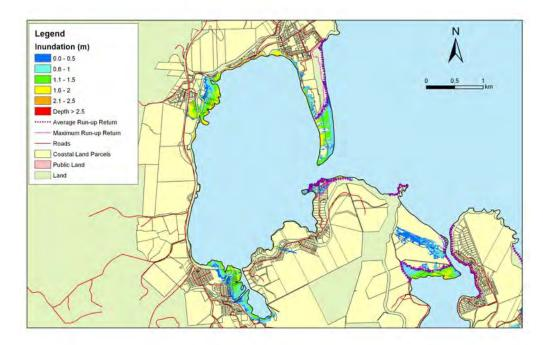
**Figure 5.144:** Warrington and Blueskin Bay - 1:500 year sea level event at MLOS + 0.5m: Maximum water depth for inundated land and the mean and maximum wave run-up
