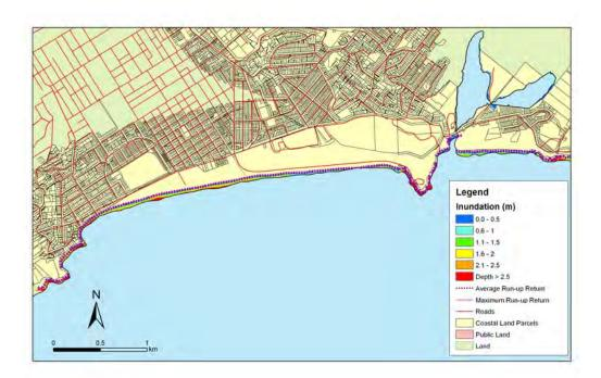
**Figure 5.103:** South Dunedin - 1:100 year sea level event at MLOS + 0.3m: Maximum water depth for inundated land and the mean and maximum wave run-up.
