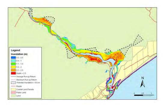
**Figure 5.56:** Toko Mouth - 1:500 year sea level event at MLOS + 0.3m: Maximum water depth for inundated land and the mean and maximum wave run-up.
