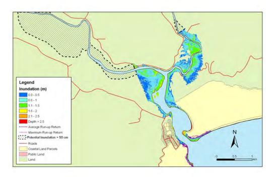
**Figure 5.22:** Papatowai - 1:50 year sea level event at MLOS + 0.5m: Maximum water depth for inundated land and the mean and maximum wave run-up.
