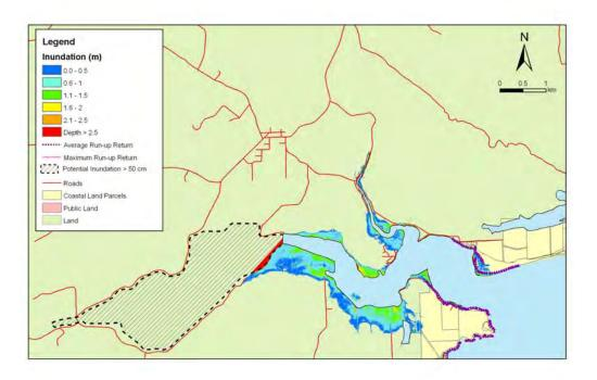
**Figure 5.31:** Catlins - 1:100 year sea level event at MLOS + 0.3m: Maximum water depth for inundated land and the mean and maximum wave run-up.
