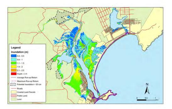
**Figure 5.149:** Karitane - 1:20 year sea level event at MLOS + 0.3m: Maximum water depth for inundated land and the mean and maximum wave run-up.
