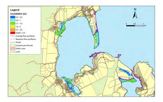
**Figure 5.140:** Warrington and Blueskin Bay - 1:500 year sea level event at MLOS + 0.3m: Maximum water depth for inundated land and the mean and maximum wave run-up.
