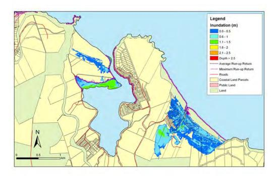
**Figure 5.128:** Long Beach and Purakanui - 1:500 year sea level event at MLOS + 0.3m: Maximum water depth for inundated land and the mean and maximum wave run-up.
