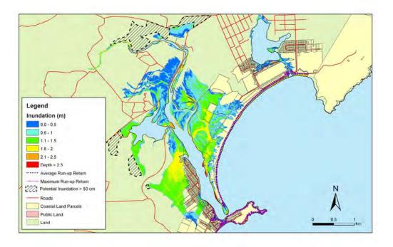
**Figure 5.150:** Karitane - 1:50 year sea level event at MLOS + 0.3m: Maximum water depth for inundated land and the mean and maximum wave run-up.
