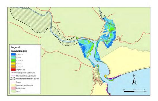
**Figure 5.20:** Papatowai - 1:500 year sea level event at MLOS + 0.3m: Maximum water depth for inundated land and the mean and maximum wave run-up.
