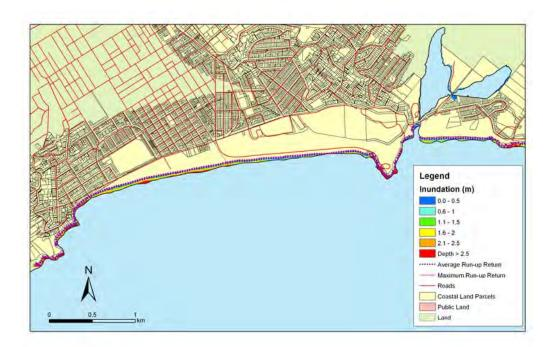
**Figure 5.105:** South Dunedin - 1:20 year sea level event at MLOS + 0.5m: Maximum water depth for inundated land and the mean and maximum wave run-up.
