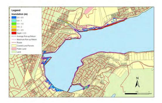
**Figure 5.118:** Dunedin Harbour - 1:50 year sea level event at MLOS + 0.5m: Maximum water depth for inundated land and the mean and maximum wave run-up.
