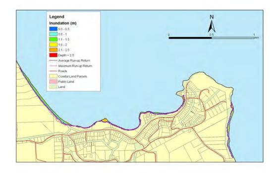
**Figure 5.168:** Moeraki - 1:500 year sea level event at MLOS + 0.5m: Maximum water depth for inundated land and the mean and maximum wave run-up
