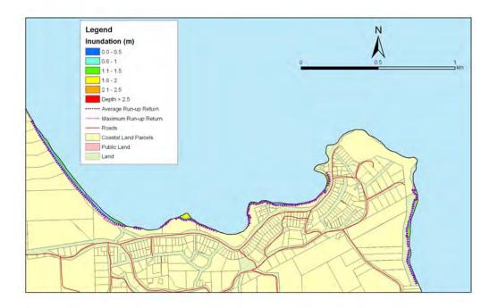
**Figure 5.161:** Moeraki - 1:20 year sea level event at MLOS + 0.3m: Maximum water depth for inundated land and the mean and maximum wave run-up.
