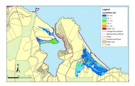
**Figure 5.129:** Long Beach and Purakanui - 1:20 year sea level event at MLOS + 0.5m: Maximum water depth for inundated land and the mean and maximum wave run-up.
