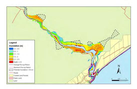
**Figure 5.57:** Toko Mouth - 1:20 year sea level event at MLOS + 0.5m: Maximum water depth for inundated land and the mean and maximum wave run-up.
