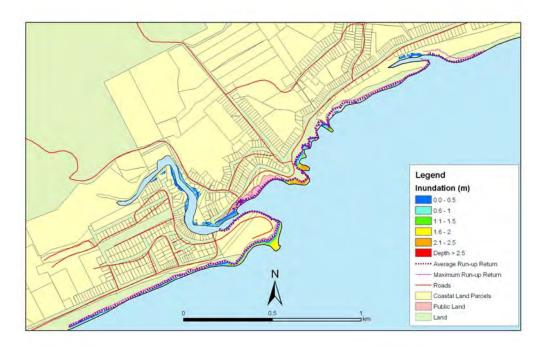
**Figure 5.73:** Brighton - 1:20 year sea level event at present MLOS: Maximum water depth for inundated land and the mean and maximum wave run-up.
