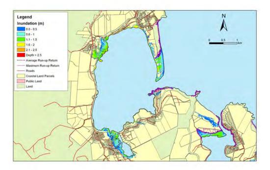
**Figure 5.142:** Warrington and Blueskin Bay - 1:50 year sea level event at MLOS + 0.5m: Maximum water depth for inundated land and the mean and maximum wave run-up.
