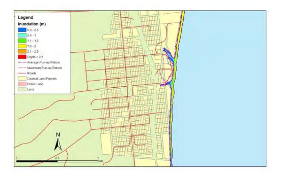
Figure 5.170: Hampden - 1:50 year sea level event at present MLOS: Maximum water depth for inundated land and the mean and maximum wave run-up.
