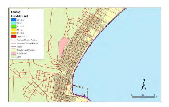
Figure 5.196: Oamaru - 1:500 year sea level event at present MLOS: Maximum water depth for inundated land and the mean and maximum wave run-up.
