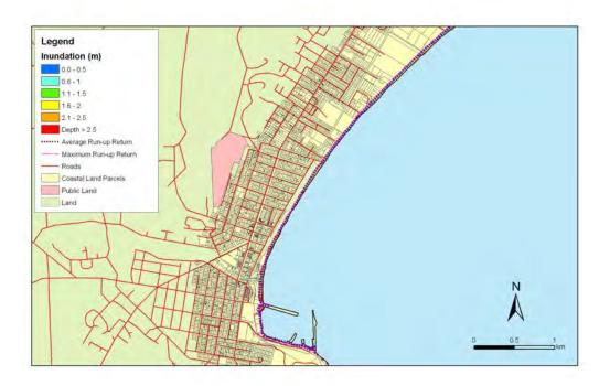
**Figure 5.201:** Oamaru - 1:20 year sea level event at MLOS + 0.5m: Maximum water depth for inundated land and the mean and maximum wave run-up.
