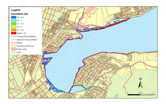
**Figure 5.119:** Dunedin Harbour - 1:100 year sea level event at MLOS + 0.5m: Maximum water depth for inundated land and the mean and maximum wave run-up.
