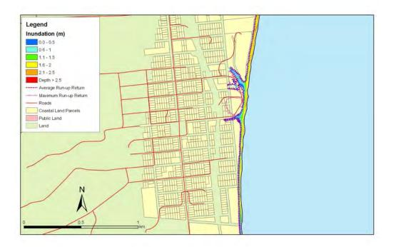
**Figure 5.172:** Hampden - 1:500 year sea level event at present MLOS: Maximum water depth for inundated land and the mean and maximum wave run-up.
