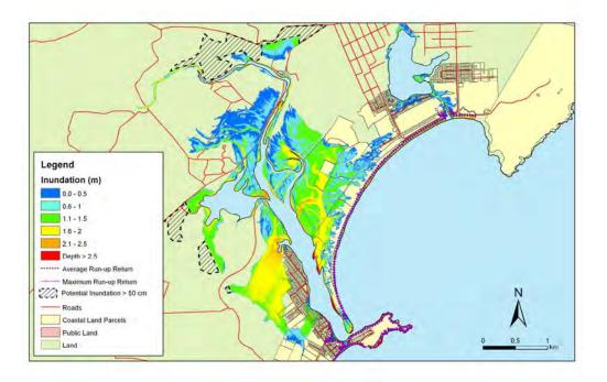
**Figure 5.152:** Karitane - 1:500 year sea level event at MLOS + 0.3m: Maximum water depth for inundated land and the mean and maximum wave run-up.
