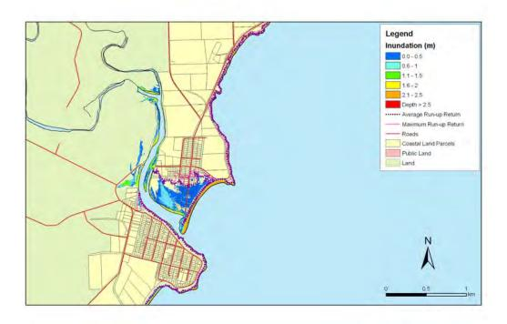
**Figure 5.183:** Taranui and Kakanui - 1:100 year sea level event at present MLOS: Maximum water depth for inundated land and the mean and maximum wave run-up.
