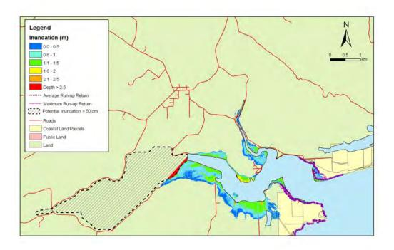
**Figure 5.32:** Catlins - 1:500 year sea level event at MLOS + 0.3m: Maximum water depth for inundated land and the mean and maximum wave run-up.
