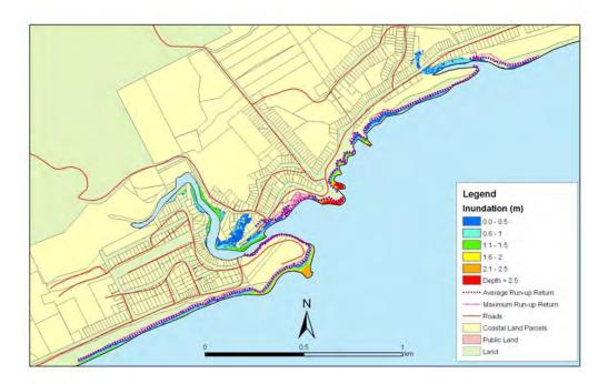
**Figure 5.83:** Brighton - 1:100 year sea level event at MLOS + 0.5m: Maximum water depth for inundated land and the mean and maximum wave run-up.
