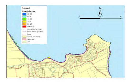
**Figure 5.165:** Moeraki - 1:20 year sea level event at MLOS + 0.5m: Maximum water depth for inundated land and the mean and maximum wave run-up.
