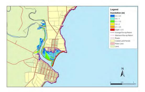
**Figure 5.192:** Taranui and Kakanui - 1:500 year sea level event at MLOS + 0.5m: Maximum water depth for inundated land and the mean and maximum wave run-up
