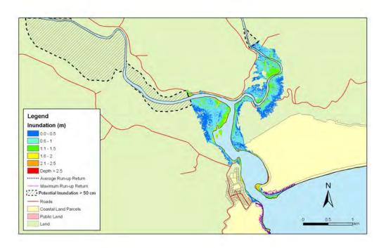
**Figure 5.21:** Papatowai - 1:20 year sea level event at MLOS + 0.5m: Maximum water depth for inundated land and the mean and maximum wave run-up.
