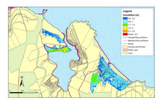
**Figure 5.132:** Long Beach and Purakanui - 1:500 year sea level event at MLOS + 0.5m: Maximum water depth for inundated land and the mean and maximum wave run-up.
