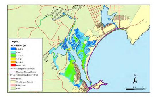
**Figure 5.145:** Karitane - 1:20 year sea level event at present MLOS: Maximum water depth for inundated land and the mean and maximum wave run-up.
