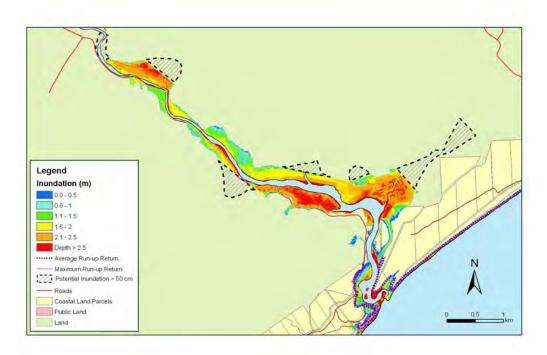
**Figure 5.59.:** Toko Mouth - 1:100 year sea level event at MLOS + 0.5m: Maximum water depth for inundated land and the mean and maximum wave run-up.
