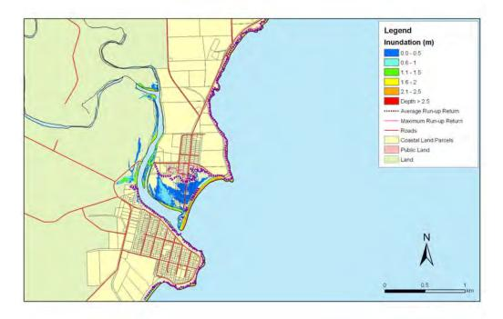
**Figure 5.190:** Taranui and Kakanui - 1:50 year sea level event at MLOS + 0.5m: Maximum water depth for inundated land and the mean and maximum wave run-up.
