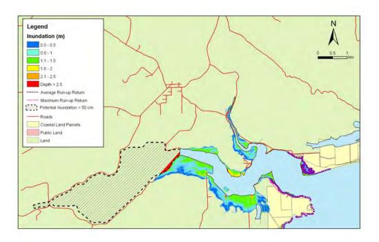
**Figure 5.35:** Catlins - 1:100 year sea level event at MLOS + 0.5m: Maximum water depth for inundated land and the mean and maximum wave run-up.
