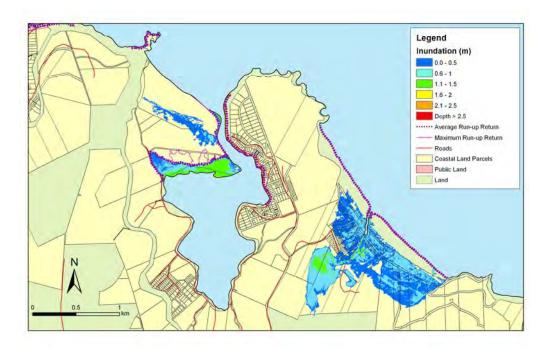
**Figure 5.130:** Long Beach and Purakanui - 1:50 year sea level event at MLOS + 0.5m: Maximum water depth for inundated land and the mean and maximum wave run-up.
