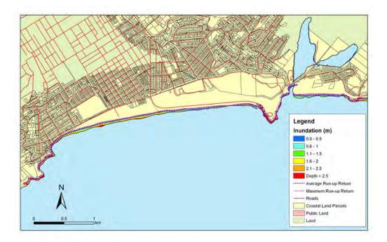
**Figure 5.101:** South Dunedin - 1:20 year sea level event at MLOS + 0.3m: Maximum water depth for inundated land and the mean and maximum wave run-up.
