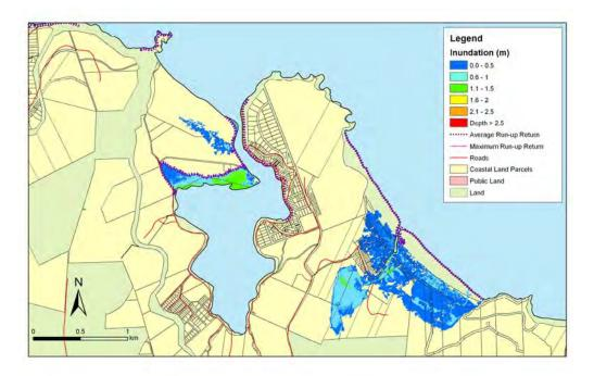
**Figure 5.127:** Long Beach and Purakanui - 1:100 year sea level event at MLOS + 0.3m: Maximum water depth for inundated land and the mean and maximum wave run-up.
