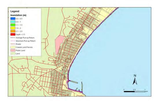
**Figure 5.200:** Oamaru - 1:500 year sea level event at MLOS + 0.3m: Maximum water depth for inundated land and the mean and maximum wave run-up.
