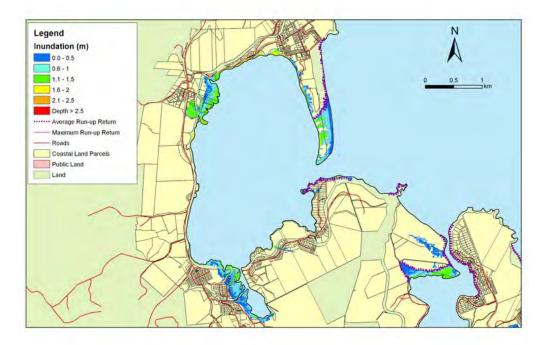
**Figure 5.139:** Warrington and Blueskin Bay - 1:100 year sea level event at MLOS + 0.3m: Maximum water depth for inundated land and the mean and maximum wave run-up.
