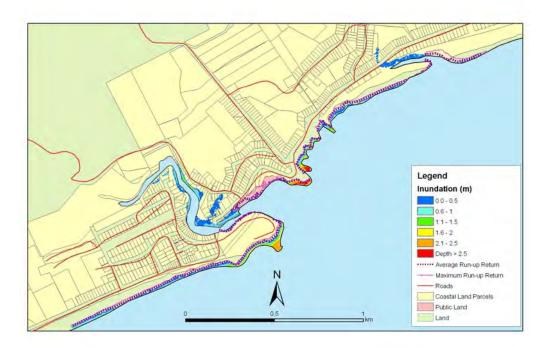
**Figure 5.77:** Brighton - 1:20 year sea level event at MLOS + 0.3m: Maximum water depth for inundated land and the mean and maximum wave run-up.
