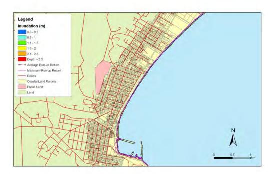
Figure 5.194: Oamaru - 1:50 year sea level event at present MLOS: Maximum water depth for inundated land and the mean and maximum wave run-up.
