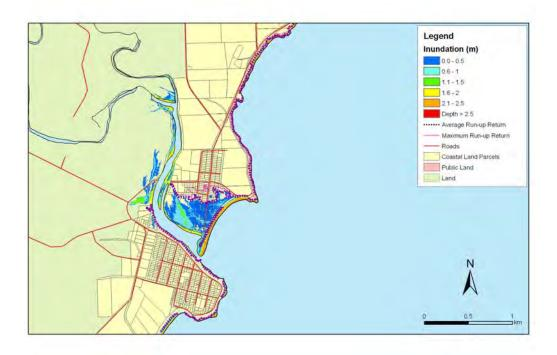
**Figure 5.185:** Taranui and Kakanui - 1:20 year sea level event at MLOS + 0.3m: Maximum water depth for inundated land and the mean and maximum wave run-up.
