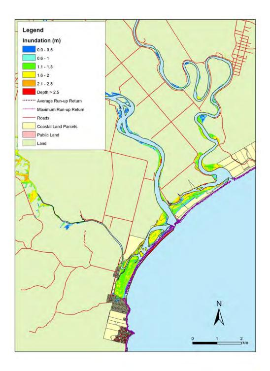
**Figure 5.44:** Kaka Point and Clutha - 1:500 year sea level event at MLOS + 0.3m: Maximum water depth for inundated land and the mean and maximum wave run-up.
