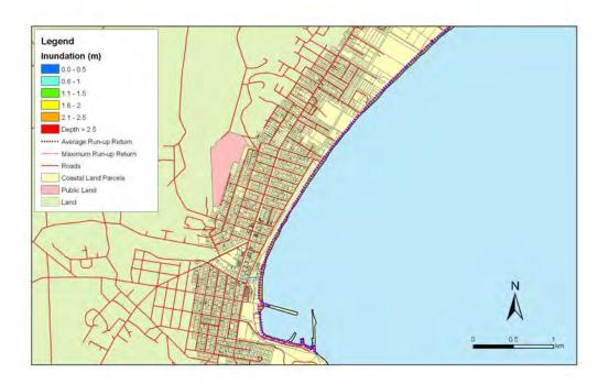
**Figure 5.197:** Oamaru - 1:20 year sea level event at MLOS + 0.3m: Maximum water depth for inundated land and the mean and maximum wave run-up.
