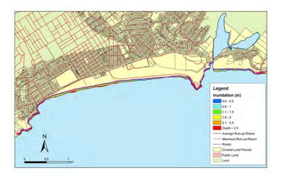
**Figure 5.107:** South Dunedin - 1:100 year sea level event at MLOS + 0.5m: Maximum water depth for inundated land and the mean and maximum wave run-up.
