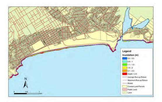
**Figure 5.108:** South Dunedin - 1:500 year sea level event at MLOS + 0.5m: Maximum water depth for inundated land and the mean and maximum wave run-up
