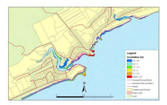
**Figure 5.81:** Brighton - 1:20 year sea level event at MLOS + 0.5m: Maximum water depth for inundated land and the mean and maximum wave run-up.
