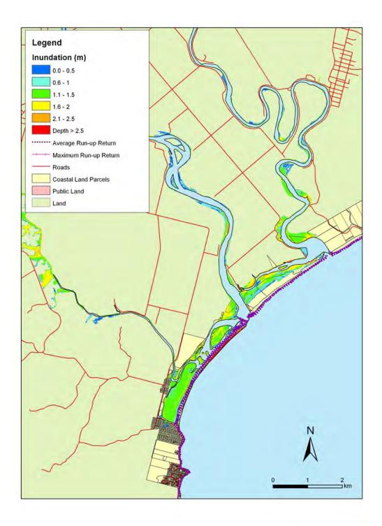
**Figure 5.42:** Kaka Point and Clutha - 1:50 year sea level event at MLOS + 0.3m: Maximum water depth for inundated land and the mean and maximum wave run-up.
