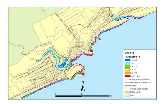
**Figure 5.84:** Brighton - 1:500 year sea level event at MLOS + 0.5m: Maximum water depth for inundated land and the mean and maximum wave run-up
