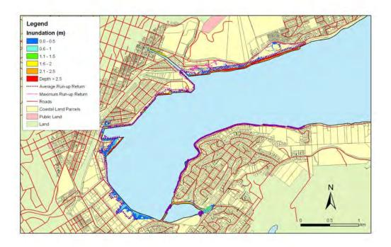
**Figure 5.117:** Dunedin Harbour - 1:20 year sea level event at MLOS + 0.5m: Maximum water depth for inundated land and the mean and maximum wave run-up.
