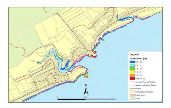
**Figure 5.78:** Brighton - 1:50 year sea level event at MLOS + 0.3m: Maximum water depth for inundated land and the mean and maximum wave run-up.
