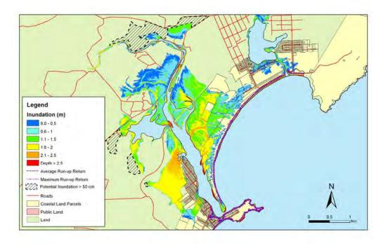
**Figure 5.156:** Karitane - 1:500 year sea level event at MLOS + 0.5m: Maximum water depth for inundated land and the mean and maximum wave run-up
