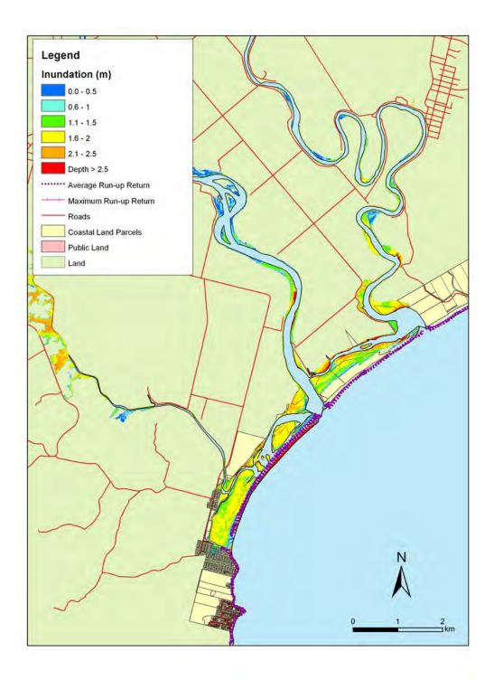
**Figure 5.48:** Kaka Point and Clutha - 1:500 year sea level event at MLOS + 0.5m: Maximum water depth for inundated land and the mean and maximum wave run-up.
