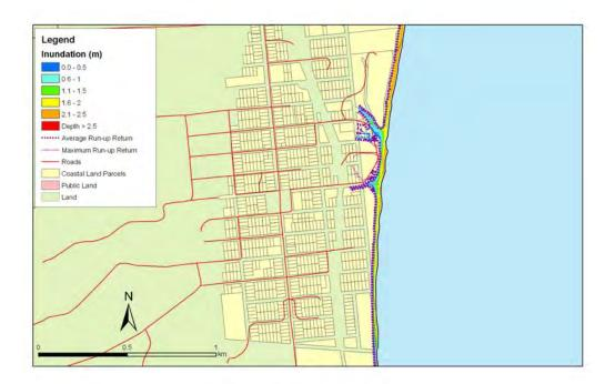
**Figure 5.173:** Hampden - 1:20 year sea level event at MLOS + 0.3m: Maximum water depth for inundated land and the mean and maximum wave run-up.
