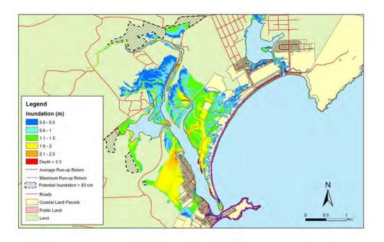
**Figure 5.154:** Karitane - 1:50 year sea level event at MLOS + 0.5m: Maximum water depth for inundated land and the mean and maximum wave run-up.
