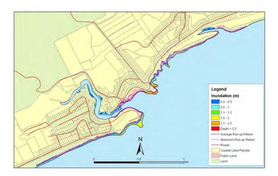
**Figure 5.75:** Brighton - 1:100 year sea level event at present MLOS: Maximum water depth for inundated land and the mean and maximum wave run-up.
