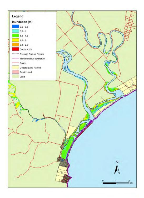
**Figure 5.41:** Kaka Point and Clutha - 1:20 year sea level event at MLOS + 0.3m: Maximum water depth for inundated land and the mean and maximum wave run-up.
