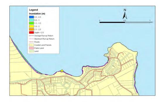
**Figure 5.162:** Moeraki - 1:50 year sea level event at MLOS + 0.3m: Maximum water depth for inundated land and the mean and maximum wave run-up.
