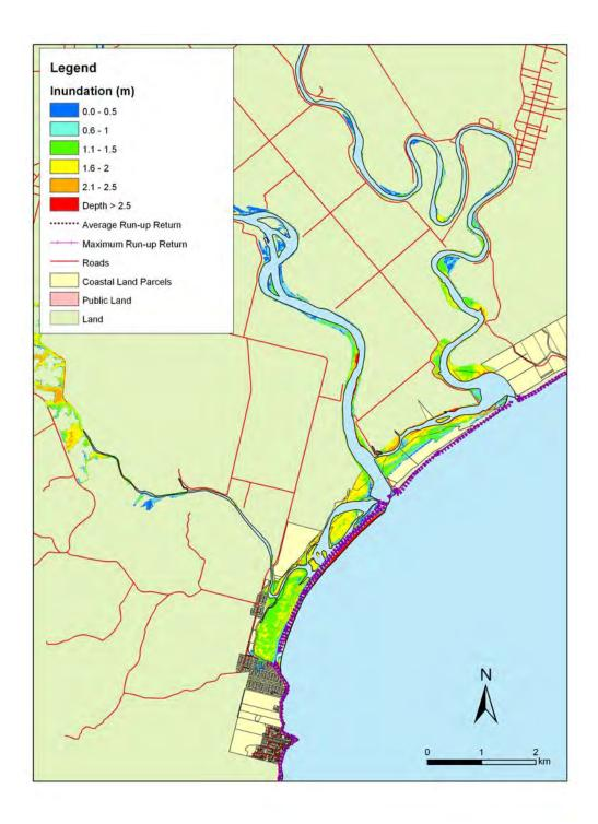
**Figure 5.46:** Kaka Point and Clutha - 1:50 year sea level event at MLOS + 0.5m: Maximum water depth for inundated land and the mean and maximum wave run-up.
