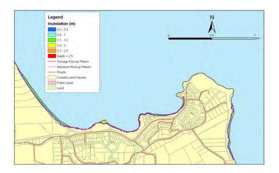
**Figure 5.167:** Moeraki - 1:100 year sea level event at MLOS + 0.5m: Maximum water depth for inundated land and the mean and maximum wave run-up.
