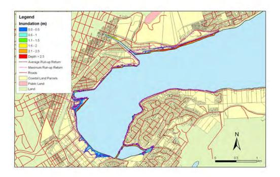
**Figure 5.115:** Dunedin Harbour - 1:100 year sea level event at MLOS + 0.3m: Maximum water depth for inundated land and the mean and maximum wave run-up.
