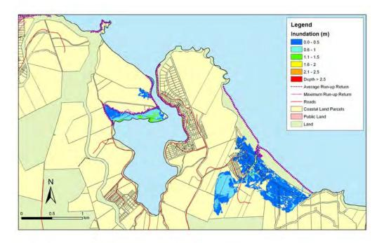
**Figure 5.125:** Long Beach and Purakanui - 1:20 year sea level event at MLOS + 0.3m: Maximum water depth for inundated land and the mean and maximum wave run-up.
