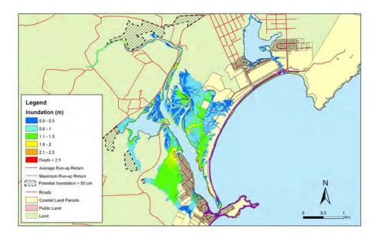
Figure 5.146: Karitane - 1:50 year sea level event at present MLOS: Maximum water depth for inundated land and the mean and maximum wave run-up.
