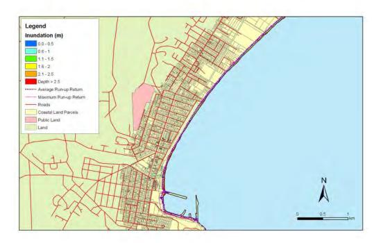
**Figure 5.203:** Oamaru - 1:100 year sea level event at MLOS + 0.5m: Maximum water depth for inundated land and the mean and maximum wave run-up.
