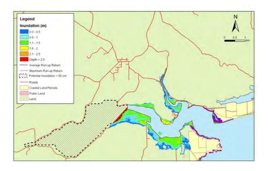
**Figure 5.36:** Catlins - 1:500 year sea level event at MLOS + 0.5m: Maximum water depth for inundated land and the mean and maximum wave run-up
