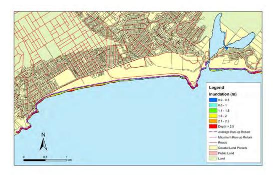
**Figure 5.106:** South Dunedin - 1:50 year sea level event at MLOS + 0.5m: Maximum water depth for inundated land and the mean and maximum wave run-up.
