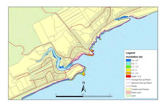
Figure 5.76: Brighton - 1:500 year sea level event at present MLOS: Maximum water depth for inundated land and the mean and maximum wave run-up.
