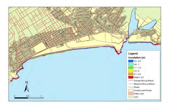
**Figure 5.102:** South Dunedin - 1:50 year sea level event at MLOS + 0.3m: Maximum water depth for inundated land and the mean and maximum wave run-up.
