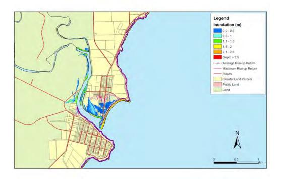
**Figure 5.181:** Taranui and Kakanui - 1:20 year sea level event at present MLOS: Maximum water depth for inundated land and the mean and maximum wave run-up.
