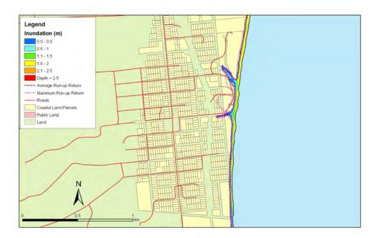
Figure 5.169: Hampden - 1:20 year sea level event at present MLOS: Maximum water depth for inundated land and the mean and maximum wave run-up.
