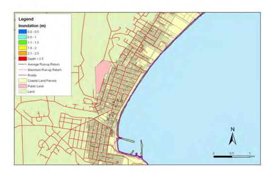
Figure 5.195: Oamaru - 1:100 year sea level event at present MLOS: Maximum water depth for inundated land and the mean and maximum wave run-up.
