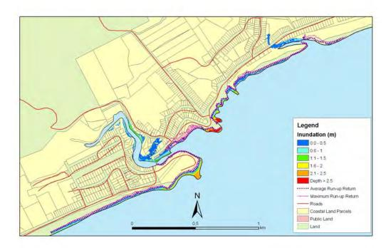
**Figure 5.79:** Brighton - 1:100 year sea level event at MLOS + 0.3m: Maximum water depth for inundated land and the mean and maximum wave run-up.
