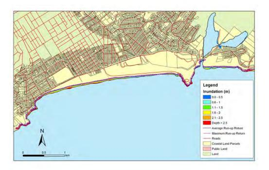
**Figure 5.104:** South Dunedin - 1:500 year sea level event at MLOS + 0.3m: Maximum water depth for inundated land and the mean and maximum wave run-up.
