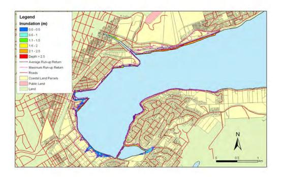
**Figure 5.113:** Dunedin Harbour - 1:20 year sea level event at MLOS + 0.3m: Maximum water depth for inundated land and the mean and maximum wave run-up.
