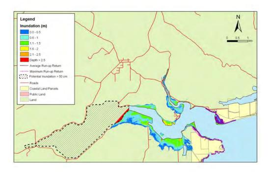
**Figure 5.34:** Catlins - 1:50 year sea level event at MLOS + 0.5m: Maximum water depth for inundated land and the mean and maximum wave run-up.
