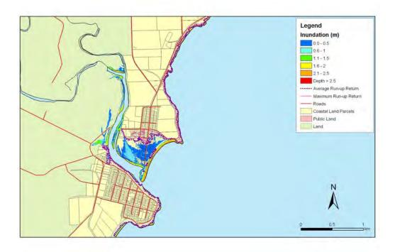
**Figure 5.191:** Taranui and Kakanui - 1:100 year sea level event at MLOS + 0.5m: Maximum water depth for inundated land and the mean and maximum wave run-up.
