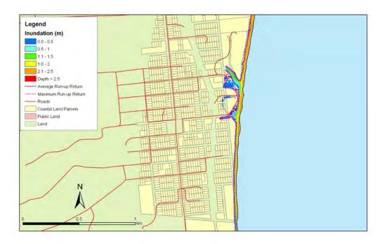
**Figure 5.178:** Hampden - 1:50 year sea level event at MLOS + 0.5m: Maximum water depth for inundated land and the mean and maximum wave run-up.
