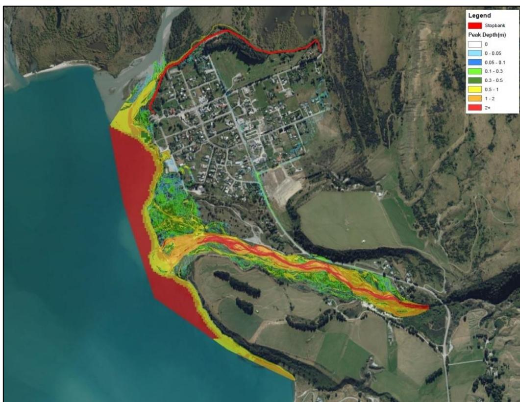
Model results showing floodwater depths for a Buckler Burn flooding scenario with a 300 m 3 /s peak flow. In this scenario minor floodwaters flow into the township area, mainly flowing northwards along Oban Street and around the eastern margin of the township.
